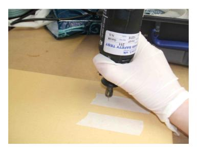
**7.** Choose suitable sized pins to hold the weight of the object, place in the holes and gently tap into the board using the small hammer.
